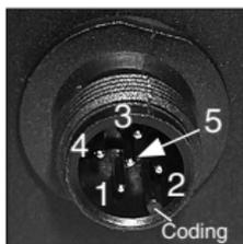
The pin assignment of the programmer is the same as the pressure switch:
