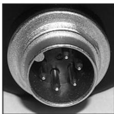
The connector plug is used for communication with a PC / laptop. The RS485 converter from KELLER (K-107 / K-104B) can be connected here.
